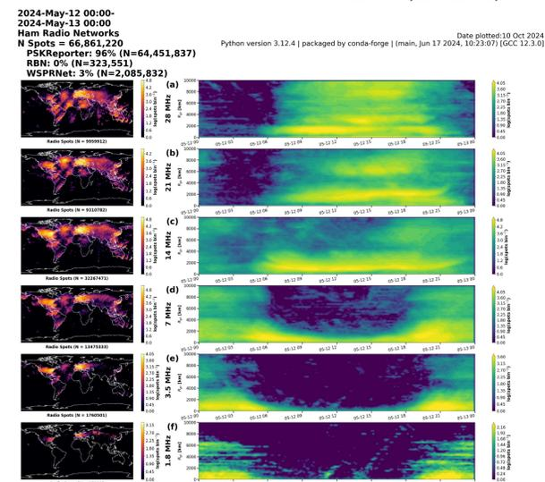
Summary figure of HF radio spots, showing radio wave propagation from 1.8 - 28 MHz over ranges of 0 - 10000 km, obtained from Amateur Radio Signal Report data during the May 2024 Gannon Superstorm.
