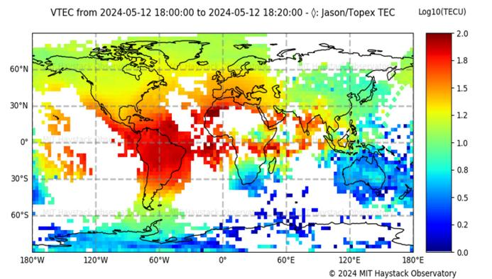
Global maps of total electron content from 6000+ ground receivers are available with resolution of 5-min in time and 1x1 degree in lat/lon, providing information about background electron density that affects propagation of radio waves at HF frequencies. This summary figure depicts a snapshot of global ionospheric conditions during the May 2024 Gannon storm.
