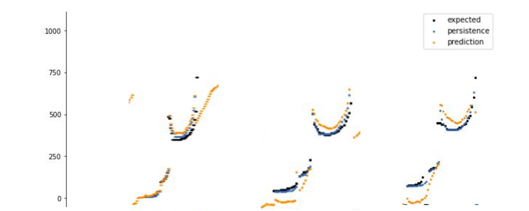
Figure 16. Sequence of predictions produced by the proposed algorithm. Each ionogram prediction is the addition of the previous prediction and the differences produced by the model.
