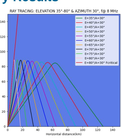
Figure 7: Ray tracing with variable elevation
