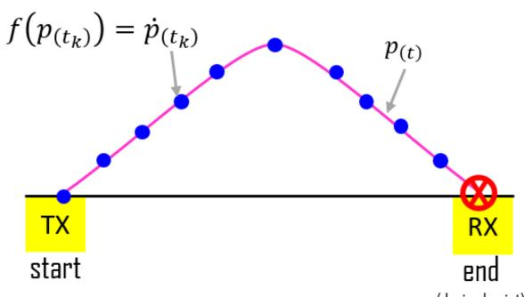
Figure 2: Collocation Method for ray tracing technique
