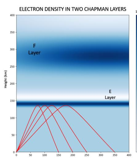
Horizontal distance (km) Figure 6: Ray Tracing, and E and F layer
