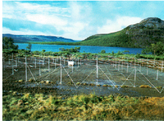
IRIS phased array riometer system at Kilpisjärvi, northern Finland
