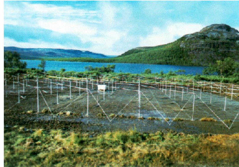
IRIS phased array riometer system at Kilpisjärvi, northern Finland
